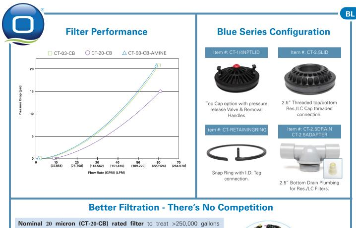
(946,353 Liters) of water @ 15 gpm (56.78 LPM) with greater than 90% reduction, estimated capacity using 2ppm of free chlorine. Nominal 3 micron (CT-03-CB) rated filter to treat >150,000 gallons
